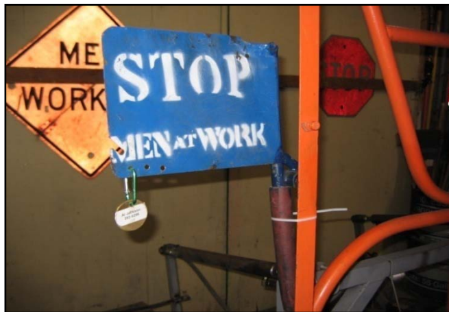
The Blue Flag protects equipment from being moved while it's being serviced.
